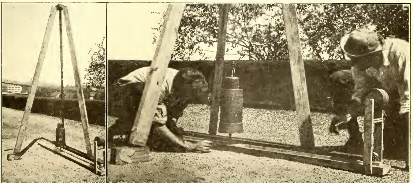
GENERAL VIEW OF SEISMOGRAPH ON POWER HOUSE ROOF AND NEAR VIEW SHOWING VIBRATION RECORD BEING TRACED ON SMOKED-GLASS PLATE
